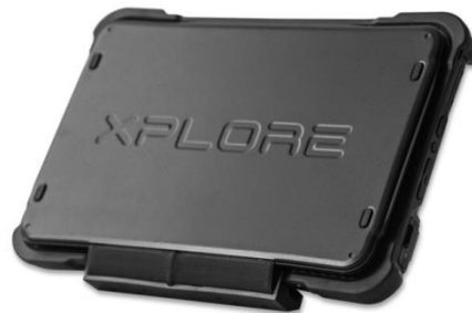
Keyboard in closed position via magnets, protecting display glass
