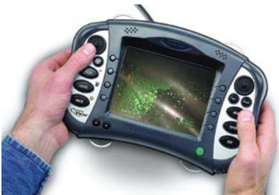
Riboflavin rinse inspection for cleaning validation
