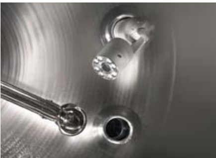
Spray ball coverage inspection for cleaning validation
