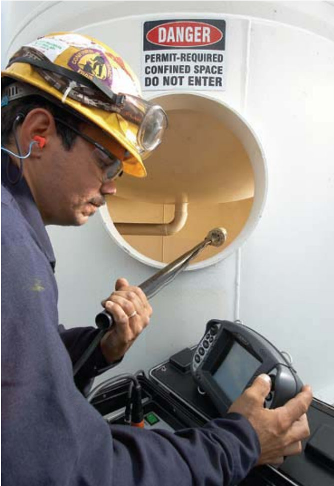
PTZ assists with confined space inspection
