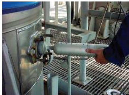
Glass-lined vessel inspection through Pharmaceutical tank inspection through 76 mm (3.0 in) \emptyset nozzle
